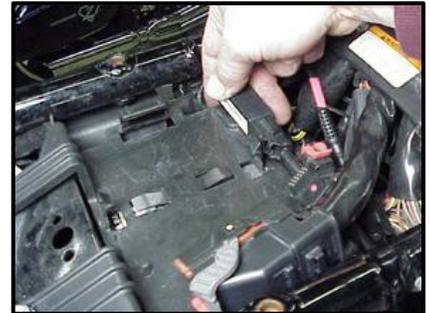
**I:** Locate the package of dielectric grease included with communication cable. Spread a small amount of grease on the AutoTune harness plug inboard of the mounting flange to allow the plug to easily slide into the ThunderMax ECM, with ThunderMax logo on harness plug facing up. Attach with screws provided.
