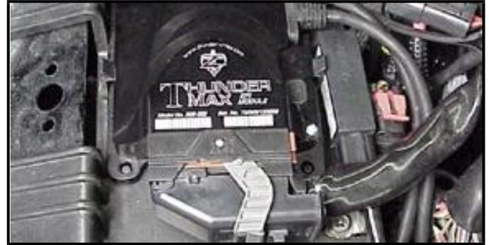
**L:** Connect the oxygen sensor harnesses to the AutoTune harness. Carefully wire tie the leads to the motorcycle. Take extra care to ensure harness and sensor leads are safe from rubbing or chaffing on the motorcycle. Use all supplied wire ties; add extra ties if needed to properly secure wiring on your installation.
