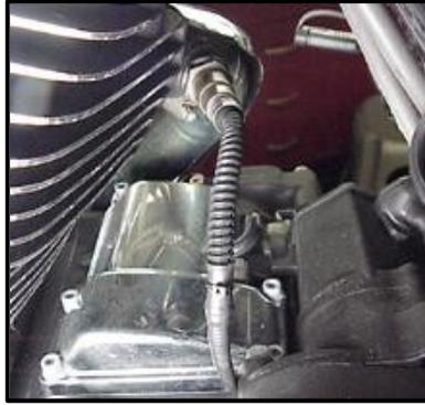
**E:** Remove factory ECM from the caddy by spreading the plastic caddy latches at the sides of the ECM. Lift the ECM up and to the right to release it from the caddy.
