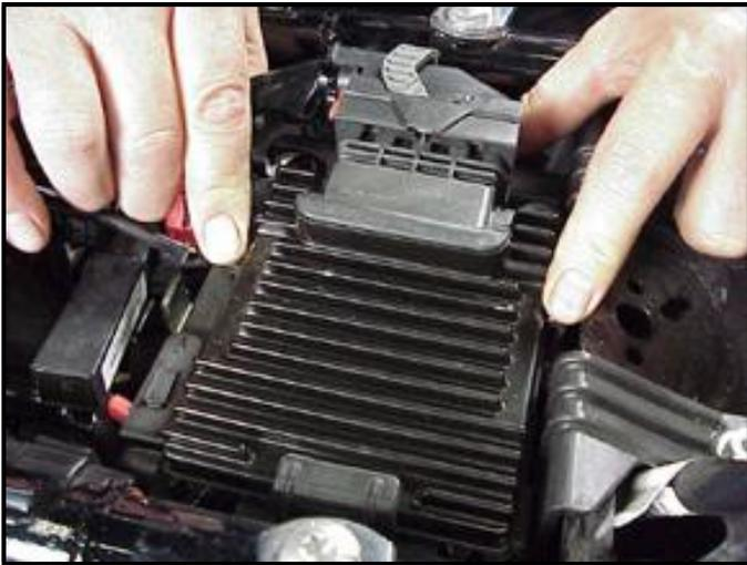
**F:** Disconnect the ECM from the connector as per the following procedure: Depress button on socket housing of the connector; rotate locking bar until it reaches the full rearward position (the index pin on locking bar will engage the rear notch in the socket housing).
